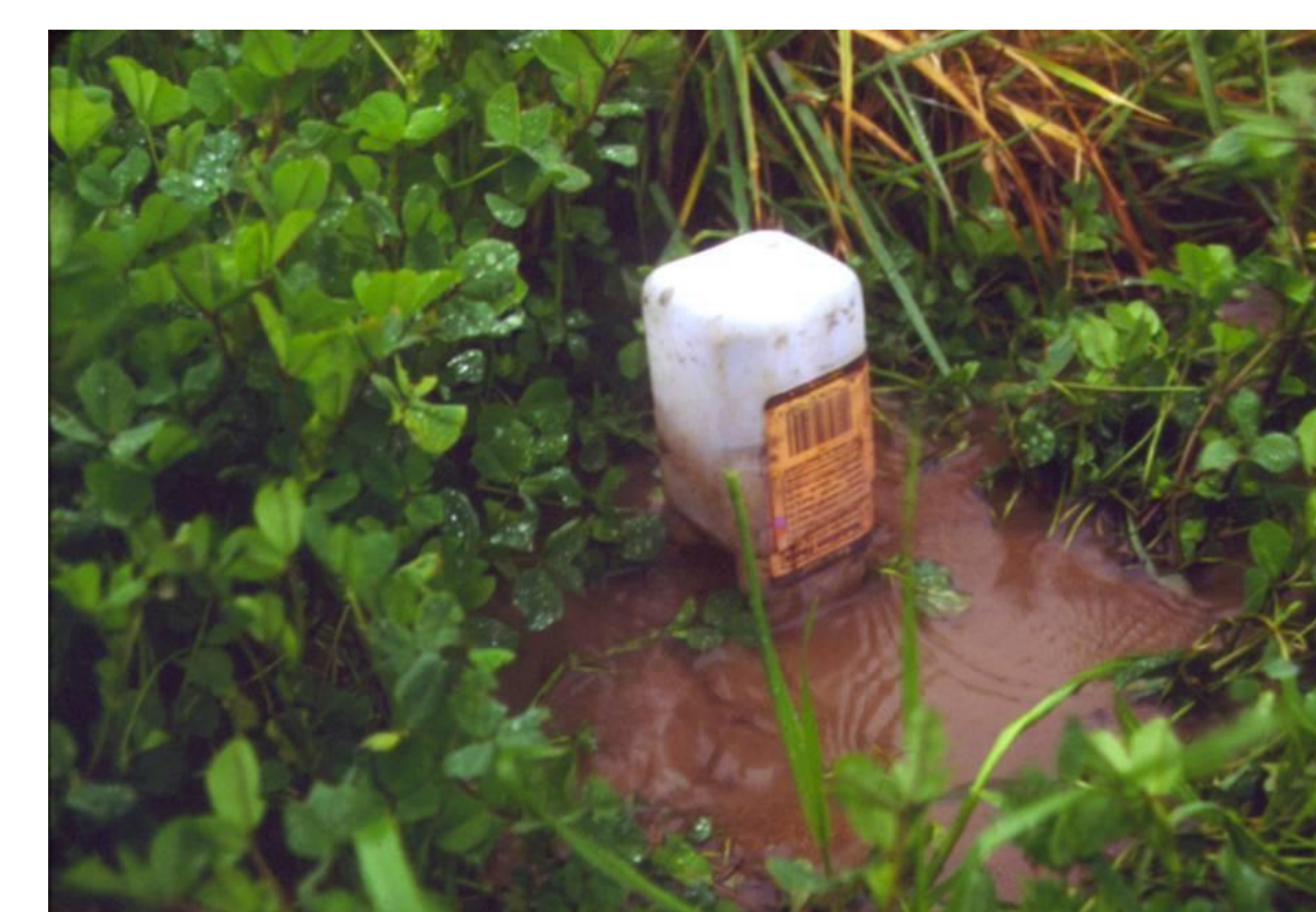
Figure 8. Sediment Capture Units designed to capture overland flow carrying sediments
