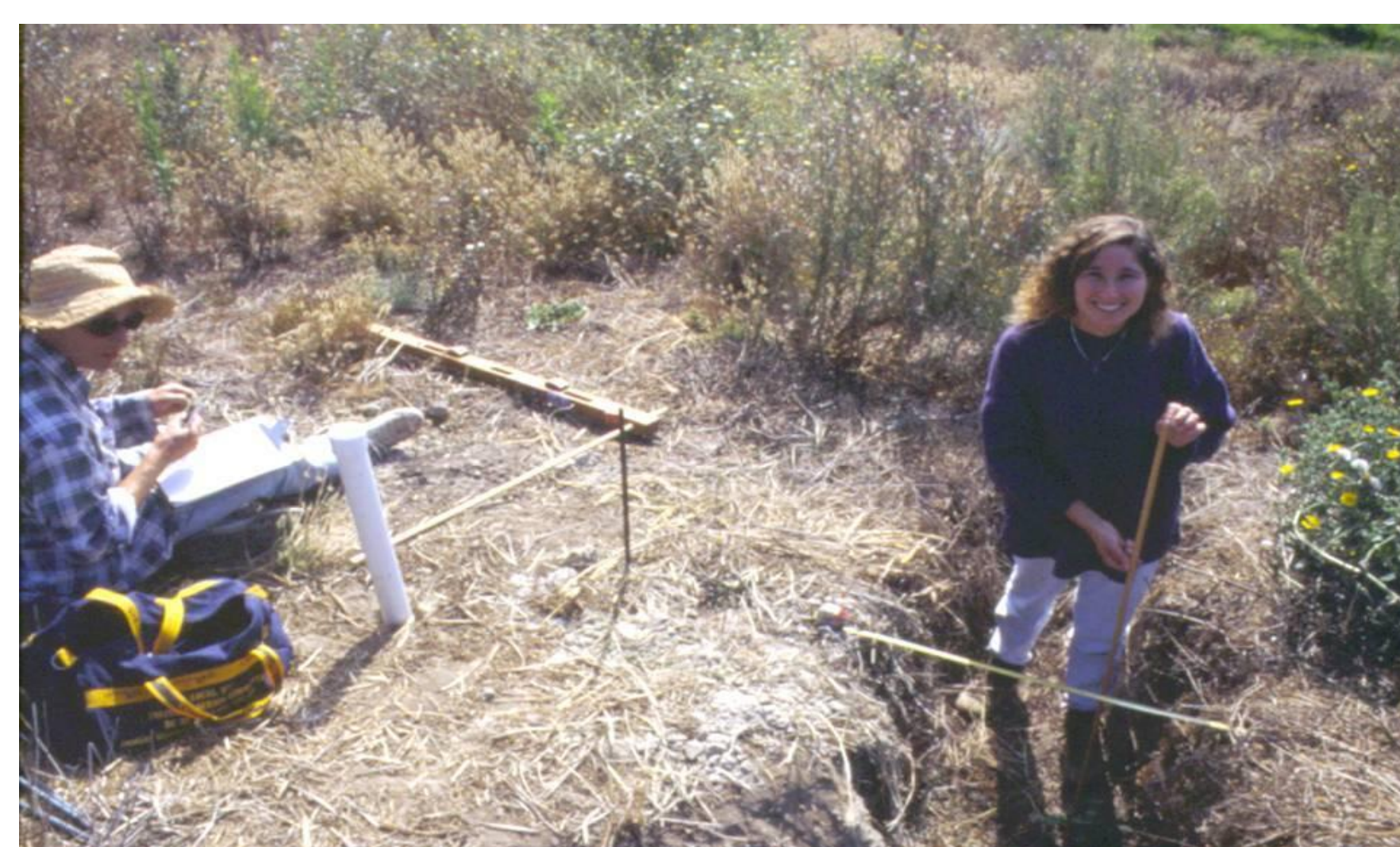
Figure 7. I am measuring gully cross section, showing decreased gully volume, due to vegetation buffers ability to capture sediment
